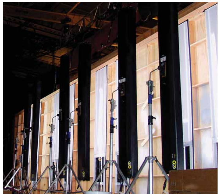
Mega 4Bank DMX fixtures (8ft), motion picture set
