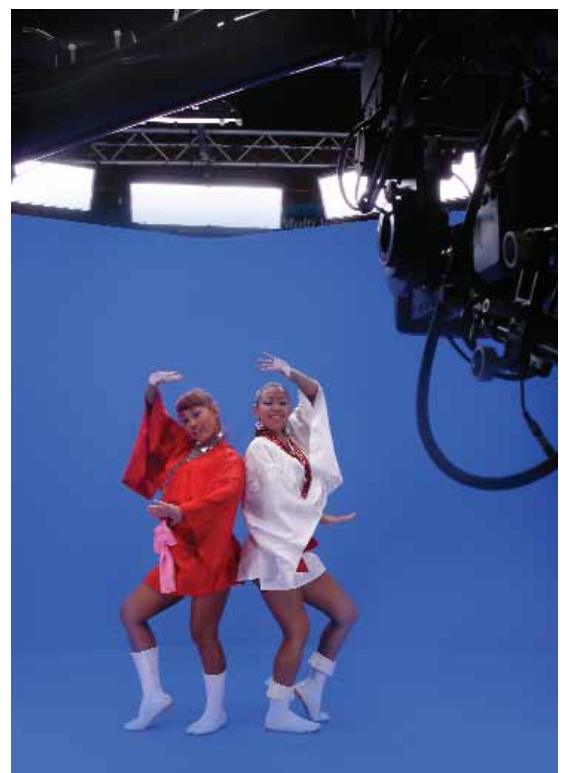
Image 45 and Image 85 DMX fixtures globed with 3200K lamps lighting virtual studio background, as well as dancers in the foreground.
